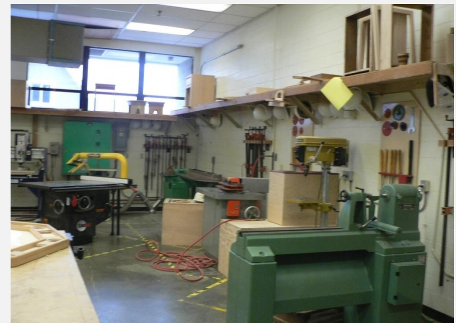
No sawdust collection at equipment
